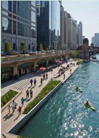
Plantings along the Chicago Riverwalk are designed for repeated and prolonged submersion.
